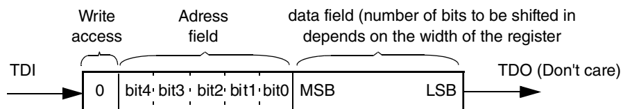
Figure 4-29. TDI/TDO on write access
